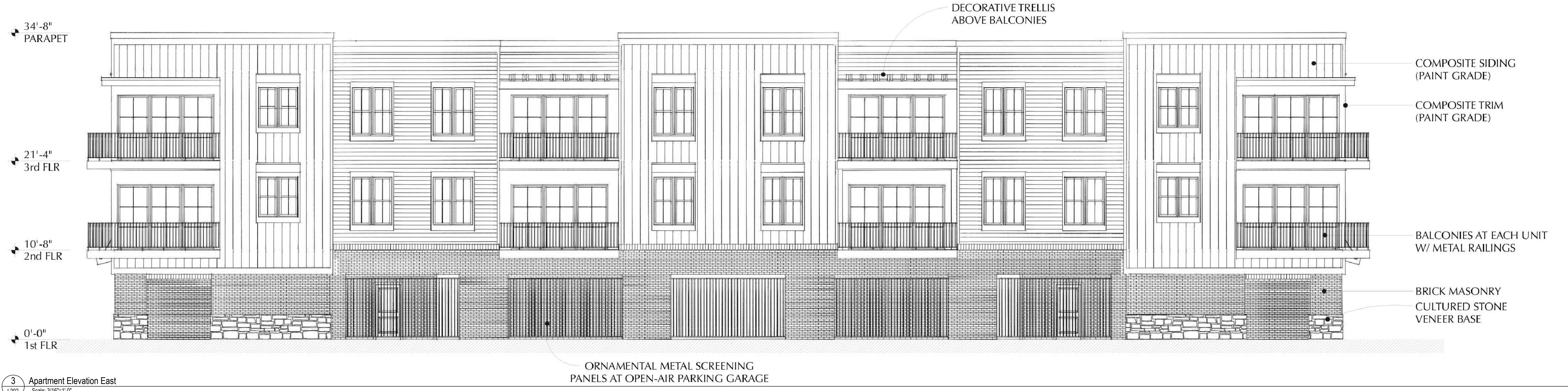
2 Apartment Elevation South (Same as North) Scale: 3/16"=1'-0"
